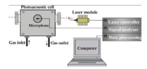
▲ "...measure the water vapour and sulphurhydrogen content of natural gas..."
